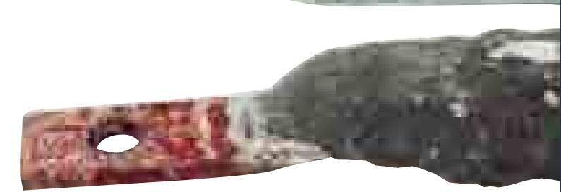
Here we can see the evidence of an efficient cathodic protection process on this completely corroded anode.
